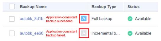
**Step 5** Return to the cloud server backup page as prompted. If the backup execution fails, rectify the fault based on the failure details shown on the page.
