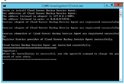
Figure 7-12 Successful client installation for Windows
